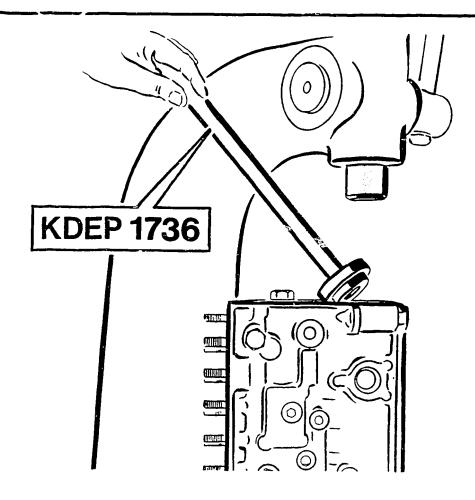
The procedure to be employed when installing the new bearing on the camshaft is the same as that used when installing the self—aligning roller bearing. The corresponding information in the repair instructions applies accordingly.
